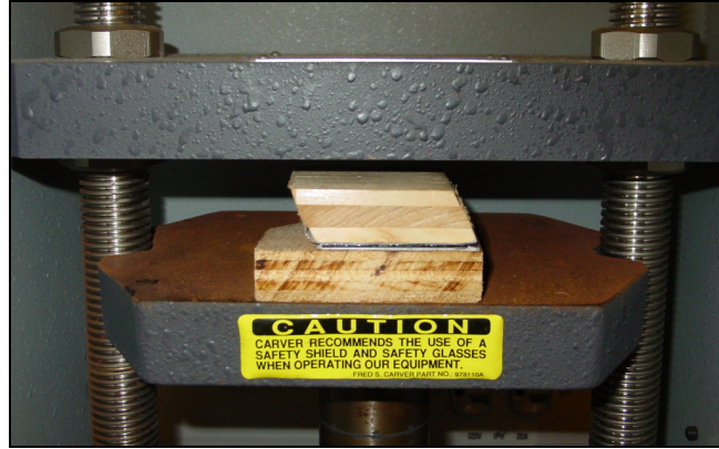
Figure 3.15 FPB sample hydraulic clamping with wooden blocks
